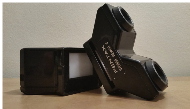
FIGURE 1. Pentax Handheld Stereo Viewer. (Pentax, Tokyo, Japan) used in study of accuracy of detecting glaucomatous progression with the traditional stereo-viewing method.
